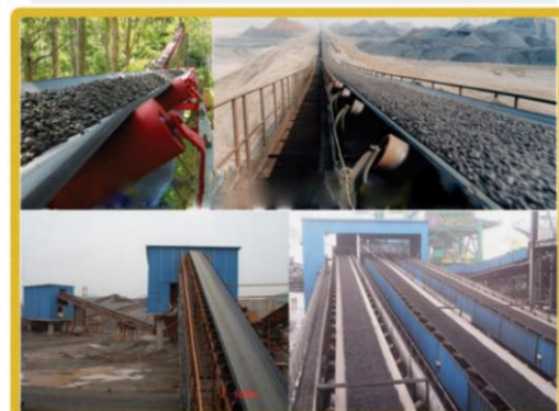
Rubber conveyor belt is suitable for transporting bulk dry granular materials, such as coal, sand, stone, cement, fertilizer
