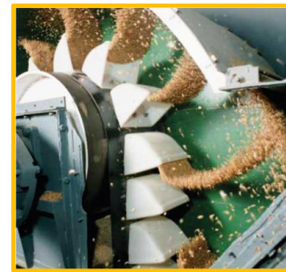
Bucket Elevator Belt
