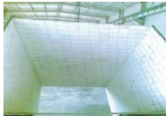
Ceramic Lined Silo
